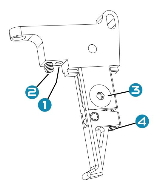
1 Preload adjustment screw: tighten the M3x12 screw to add preload, loosen the M3x12 screw to loosen preload. 🚹 Excessive high trigger preload will generate slam fire and safety issues.
